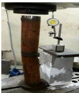
Fig -1: Control sample after fail.
