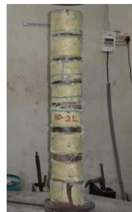
huge solidness of the AFRP holding, the section examples had the option to accept a more burden when contrasted with SHTS-HS-1L and SHTS-HS-2L. Right now, clasping of the segment examples was less significantly in the wake of intersection a definitive
